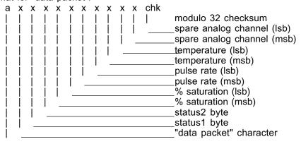
If the two temperature bytes are E\ they decode as (("E" - "@")\*32) + ("" - "@"). ("E" - "@") is equal to 5, multiplied by 32 is 160. Then add ("" - "@"), which is equal to 28, to get 188. This represents 18.8 degrees centigrade. An ACK is send upon reception of a valid command packet. A NAK is sent when something is wrong with the packet or it's contents.
