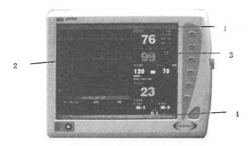
Pic 1-2 Main screen display of a portable multi-meter monitor
