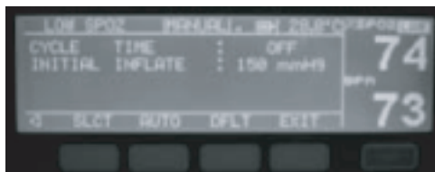
Figure 20: NIBP Cycle Time and Initial Inflate settings
